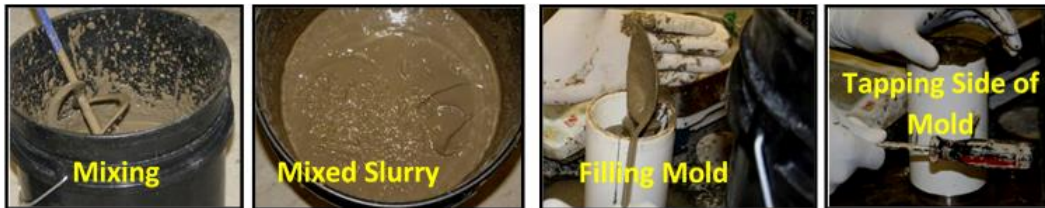
Figure 2.3 Preparing of Lightly Cemented VHMS test Specimens
